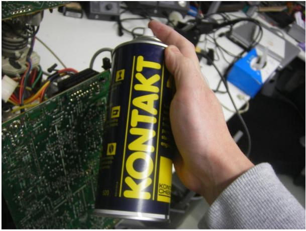
Inject contact spray into all potentiometers.
