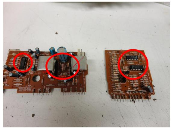
The two auxiliary boards: Stereo Amplifier and TTL-Interface. The marked parts are the most susceptible to print spot fractures.
