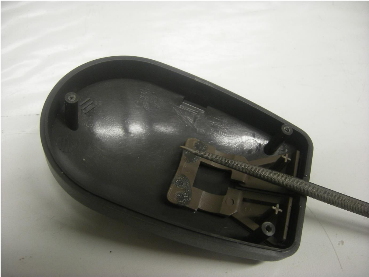
Adjusting the case for the "new" cable.
