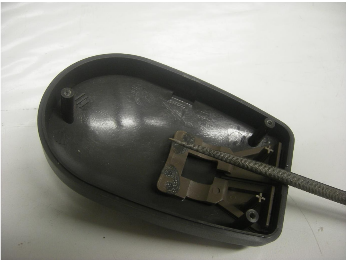
Adjusting the case for the new cable.
